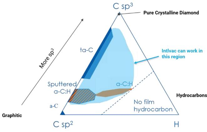
Figure 6: Phase diagram of carbon showing graphite, diamond, and hydrocarbons. Highlighted area depicts region of  $sp^2 - sp^3$  selectivity for Intlvac
