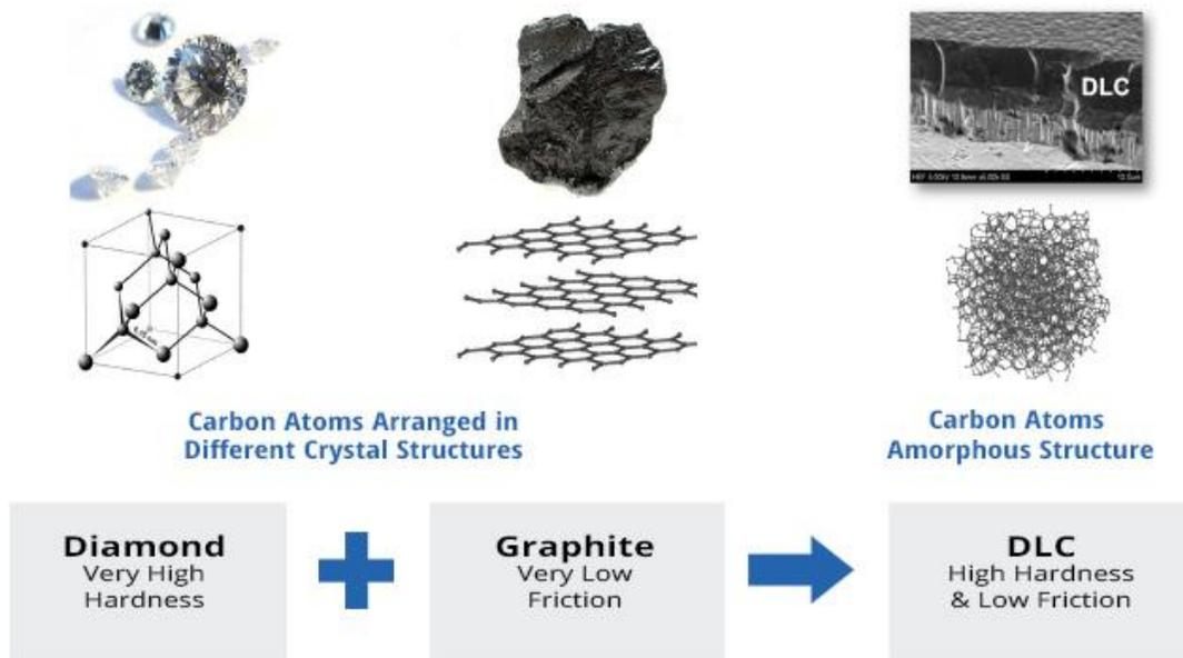
Figure 5: Diamond, Graphite, and Diamond Like Carbon traits
