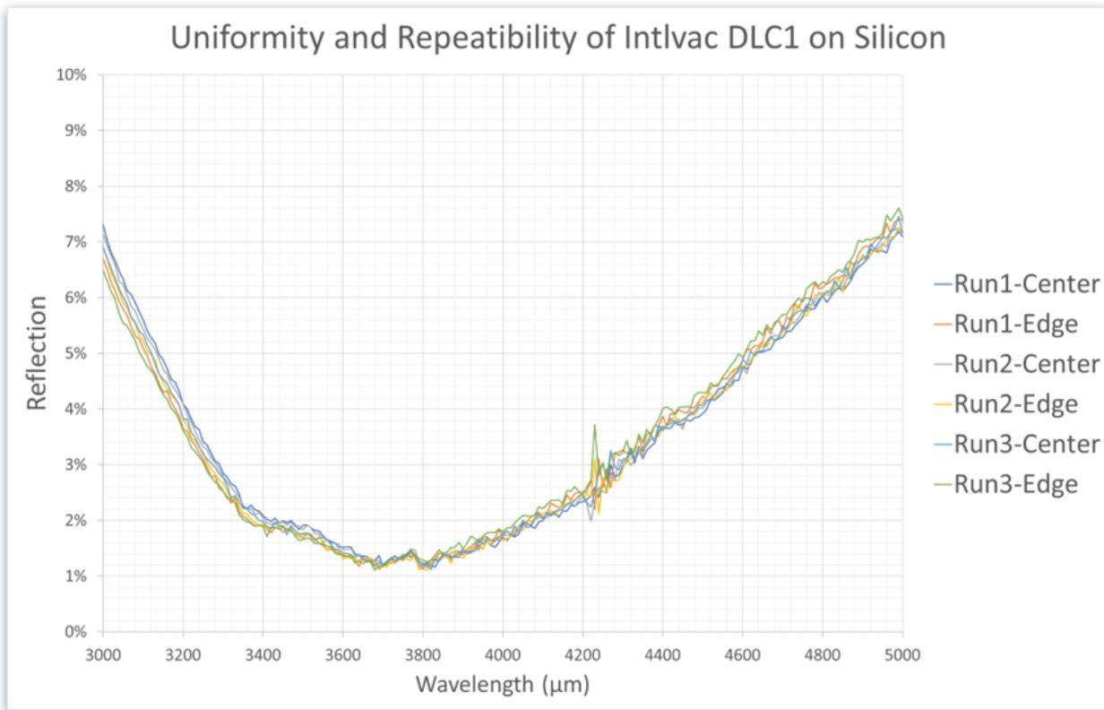
Figure 10: Graph showing uniformity and repeatability of DLC processes. Film characteristics also show remarkable performance across the entirety of the coating, a key difficulty in large area thin film coatings meant for performance.
