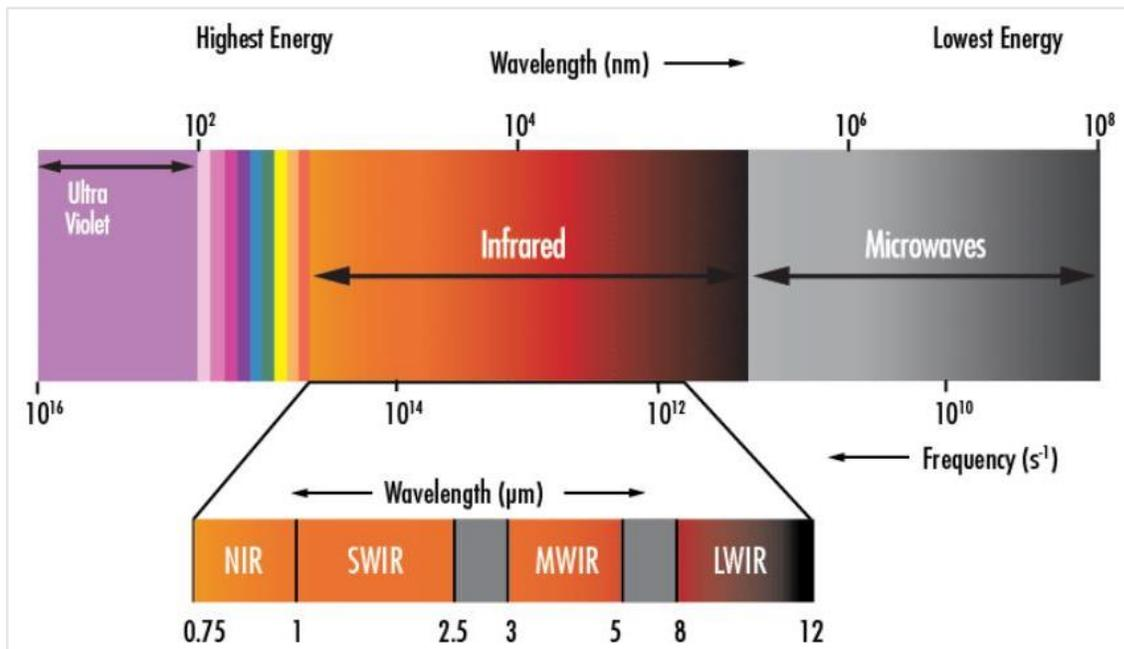
Figure 12: Electromagnetic Spectrum highlighting the IR Range. *Edmund Optics.*
