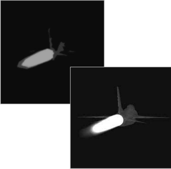
*Figure 4:* Example of high reflectance signal loss in IR.
